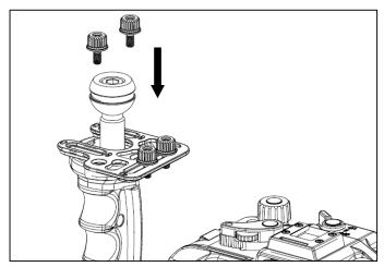
Attach the universal right handle bracket to the strobe mounting ball as shown.
