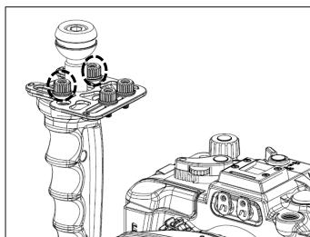
Align it to the threaded holes of #71311, and tighten by two thumb screws provided.
