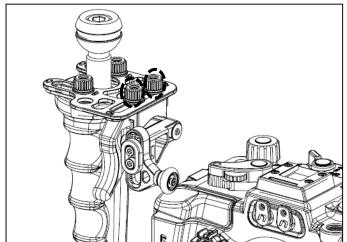
Mount the shutter release extension onto the universal right handle bracket as shown, and tighten it by the two thumb screws provided.
